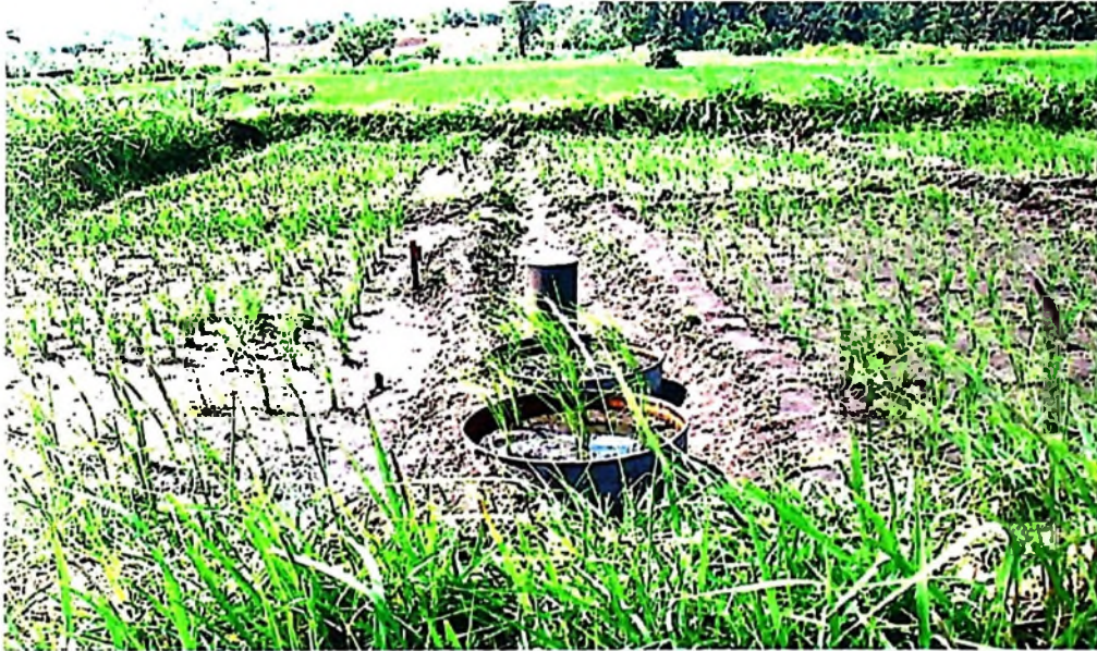
Figure 7: Picture showing the siting for one of the piezometer pipes, drainage lysimeter and a rain gauge within the experimental site
