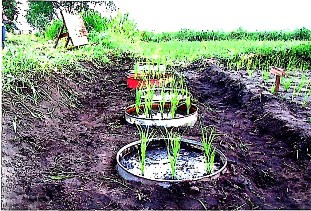
Figure 6: Three pairs of drums planted with rice being used as lysimeters
