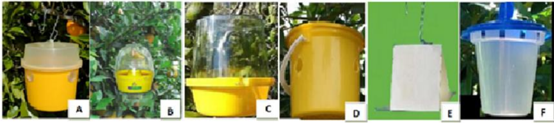
Figure 1.2: Different trapping devices : a) Tephri, b) Multilure, c) Mcphail , d) Lynfield, e) Jackson e f) Sensus. Source: Manrakhan (2010).
