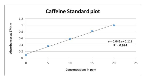
**Figure 1: Standard Calibration Curve**
