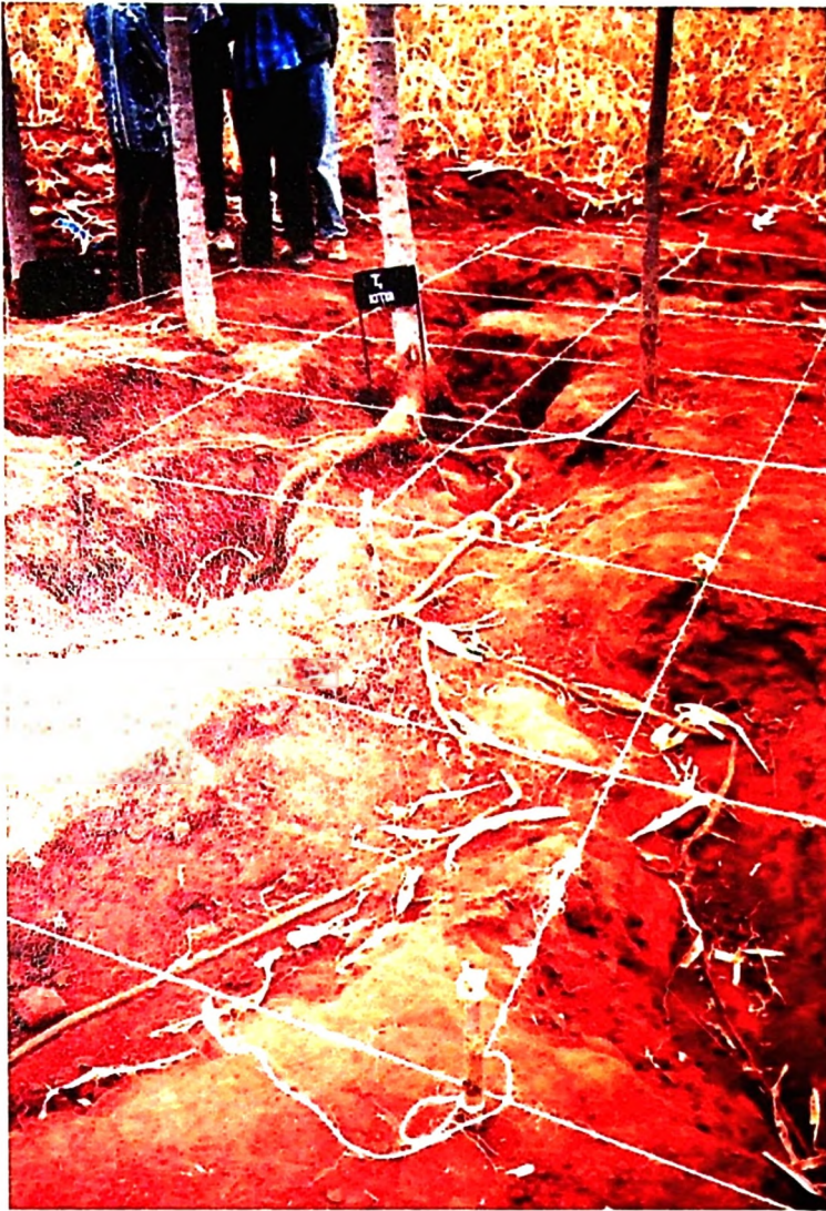
Plate 3: Root architecture of 3 year-old Melia volkensii indicating grid (1 x 1 m) used in measuring XYZ co-ordinates of root branching, bending and end events from a set origin (see Fig. 2.3.2).
