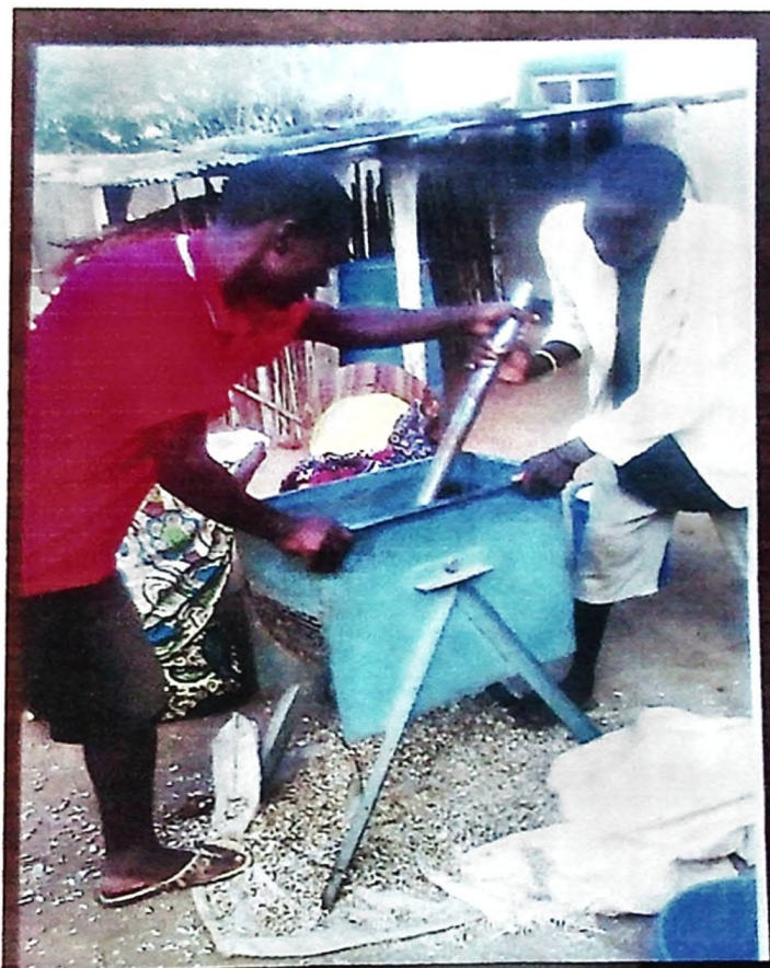
Figure 25: Hand operated sheller used to shell groundnuts in Mkalama village
