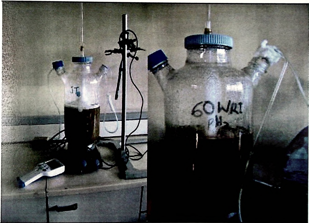
Photo 3.1: Submerged Fermentation with Belco-Micro carrier Spinner flasks.
