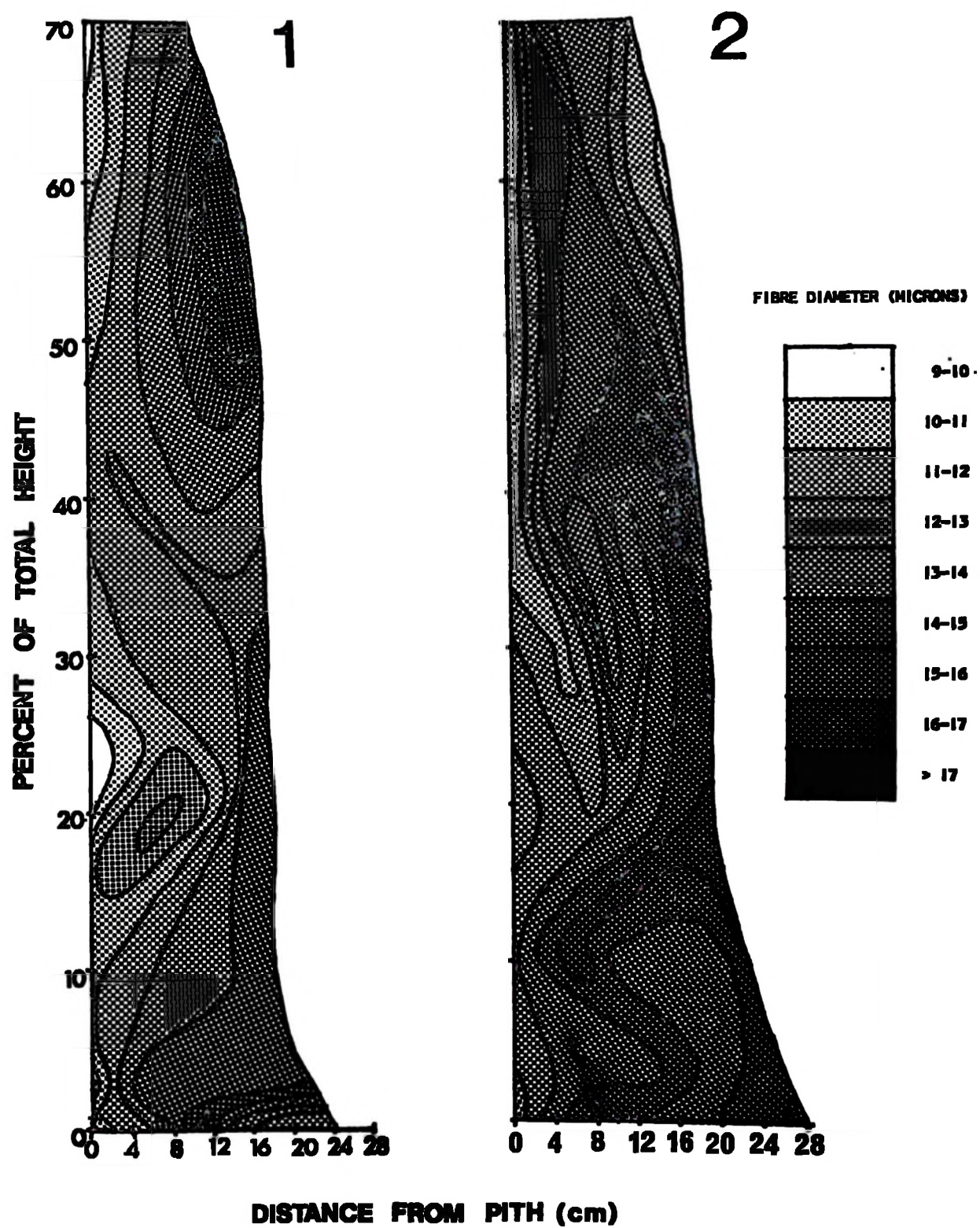
FIGURE 7.4. Variation in fibre diameter in two trees of E. deglupta
