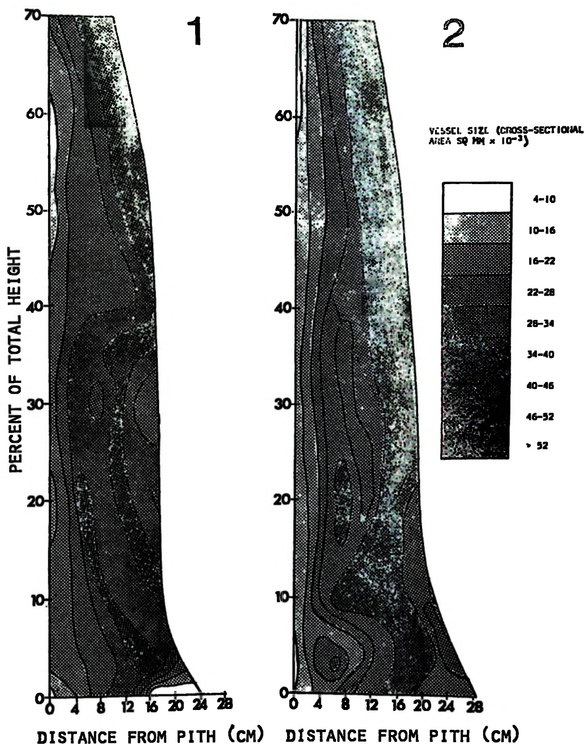
FIGURE 7.6 Variation in vessel size in two trees of E. deglupta . Size of vessels is expressed as the area of their cross-sections in units of \text{sq mm} \times 10^{-3} .
