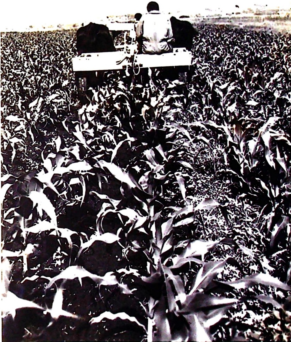
A.8.3: The UAC tool Carrier used for weeding.
