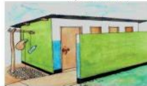
(c) Improved Pit Latrine for schools (no vent pipe)
