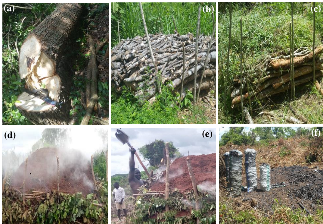
Plate 5: Charcoal making procedures in Handeni district (a) Felling the trees (b) Stacking of the logs (c) Covering with grasses (d) Covering with dump soil (e) Controlling supply of oxygen (f) Packing of charcoal.
