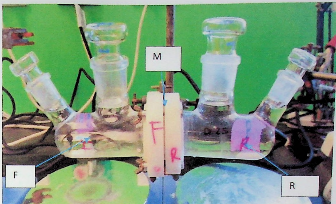
F-feed solution, M-membrane and R-receiving solution
