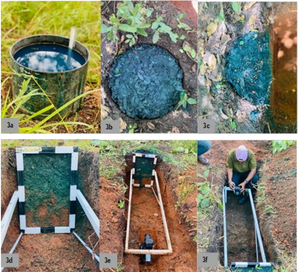
Figure 3.3: Water infiltration and pathways measurement in the field (Picture was taken by Hadija Mchelu)
