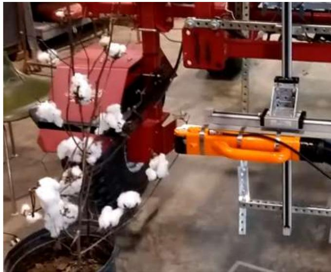
Figure 5. The end-effector comes close to the cotton bolls and sucks them using vacuum suction
