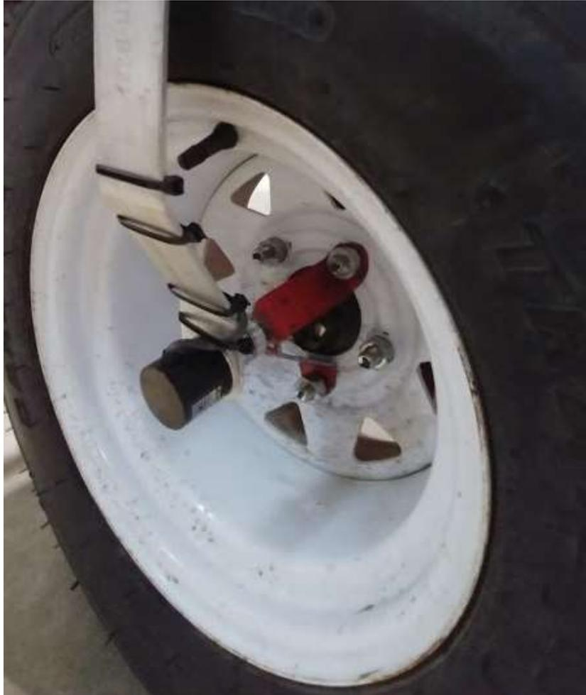
*Figure 2. Encoder installed on the front tire of the rover to give the feedback input pulses which indicates how far the rover has moved from one point to another*
