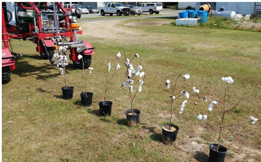
Figure 18. The experiment was set up at UGA grounds to test the robot on picking the bolls on a simulated environment consisting of six potted cotton plants
