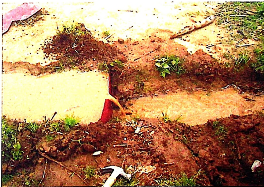
Figure 5: Flow measurement in Fuku canal using a v- notch weir
