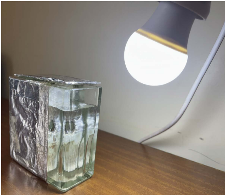
Fig 1. Hatching container for Artemia salina egg incubation.
