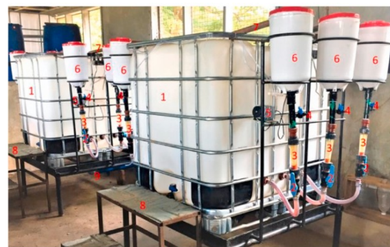
Plate 1. Side view of the experimental RAS unit used in the experiment. Showing all the functional parts of the system and water circulation was from 1, 2, 3, 6, 7 and back to 1.
