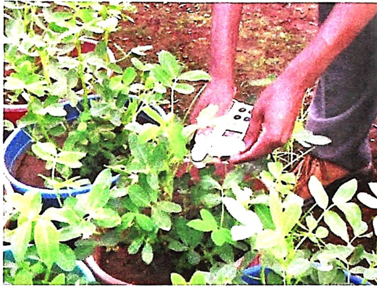
Figure 1: Recording SPAD Chlorophyll Meter Reading using SPAD Chlorophyll Meter
