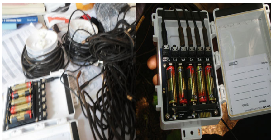
Plate 29.1 Temperature sensors and data logger
