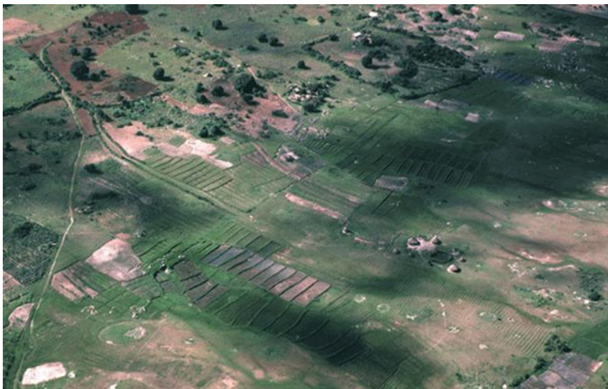
Fig. 4 View of majaluba water harvesting system. Photograph John Gowing
