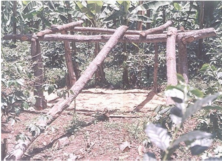
Plate 2: Traditional wooden log sawing platform (Kweka, 2007)
