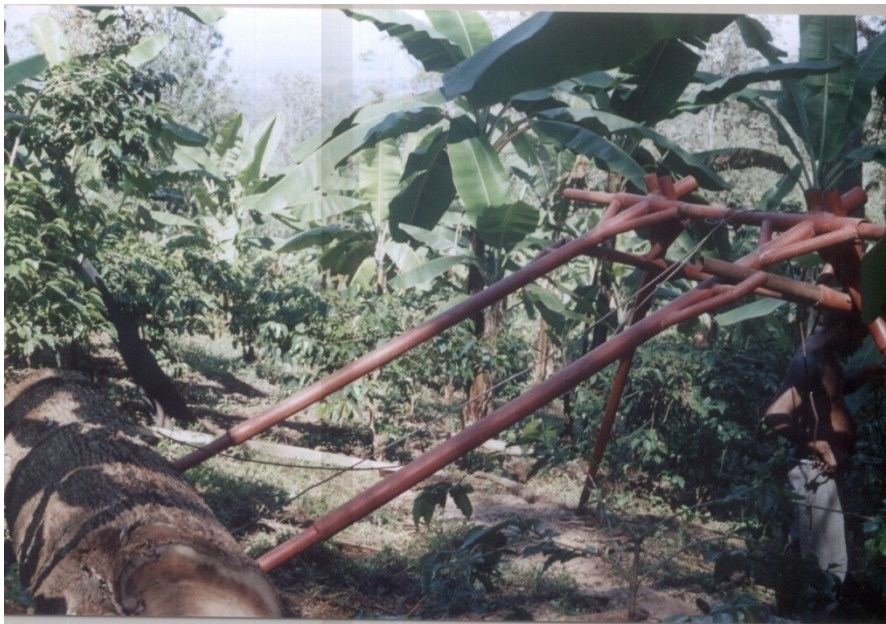
Plate 3: Portable steel log sawing platform (Kweka, 2007)
