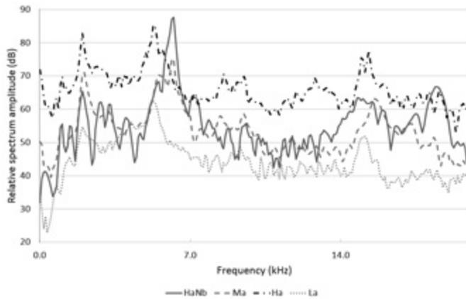
**Fig. 1.** Spectral profiles of 4 distinctive types of larval sound impulses detected in cracked corn: HaNb, solid line; Ma, dashed line, Ha, dash-dot-dotted line, and La, dotted line. Horizontal axis indicates frequency in kHz and vertical axis indicates relative spectrum amplitude in dB.
