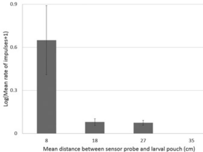
**Fig. 3.** Effects of distance on detectability of larval sound impulses. Horizontal axis indicates the mean distance between the larval pouch and the sensor; vertical axis indicates the  $\log_{10}$ -transformed mean rate of impulses detected at that distance. Bars indicate the standard error of mean transformed rate.
