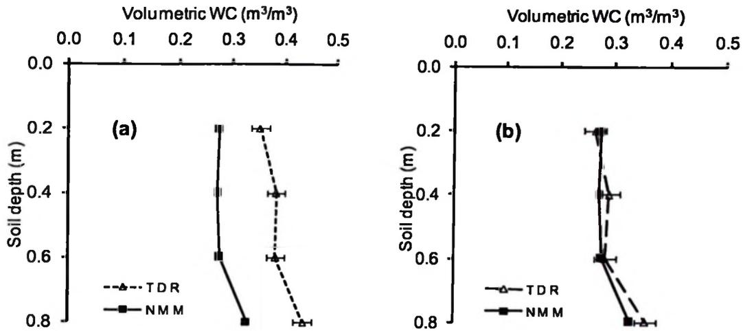
**Fig. 4.2. Comparison of TDR and NMM soil moisture measurements on the non-cover-cropped treatment at temperature ranges 8.8°C to 2.5°C on November 22, 2005: (a) before temperature correction and (b) after temperature correction. The TDR measurements were taken as average of three replicates.**
