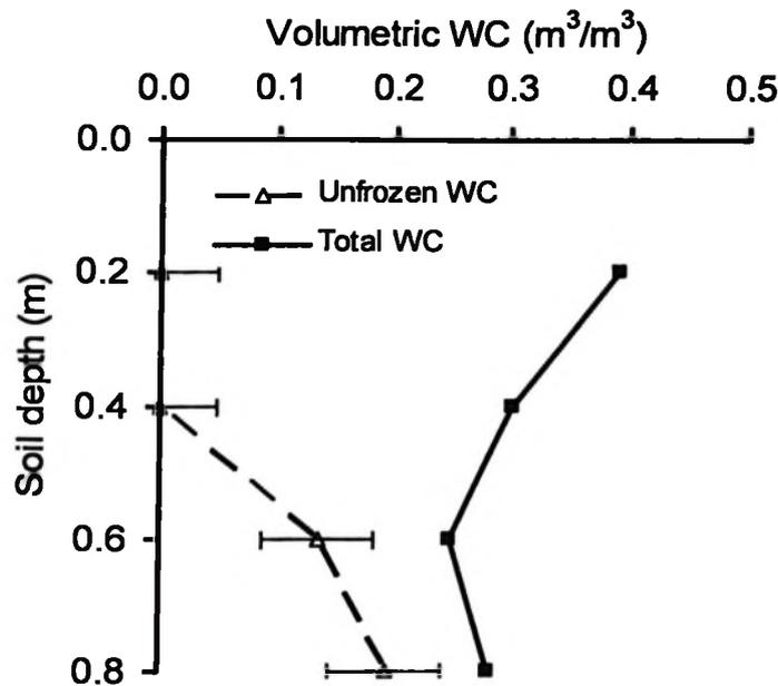
**Fig. 4.3. Variation of liquid (unfrozen) and total water content with depth for the non-cover-cropped treatment on January 30, 2006. Error bars indicate standard errors of measurements.**
