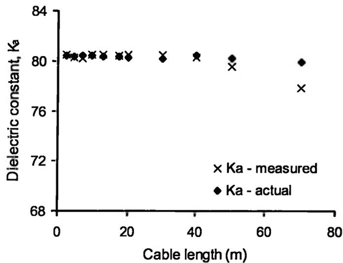
**Fig. 3.3. Comparison of the measured and the actual dielectric constants ( $K_a$  values) for water content measurement.**
