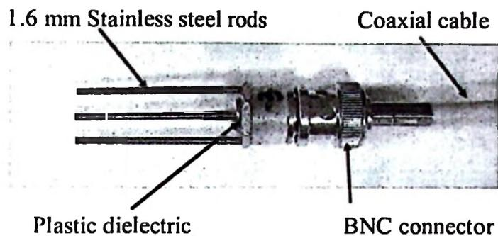
**Fig. 2.2 A typical three-wire 35 mm TDR miniprobe for water content measurements.**
