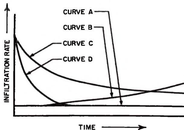
**Fig. 2.6 Schematic diagram of infiltration rates in frozen soil for different moisture conditions prior to soil freezing: (A) saturated, (B) 70-80% saturated, (C) low moisture content & high temp, and (D) low moisture content & low temp (Source: Fig. V.7 of Gray et al. 1973).**
