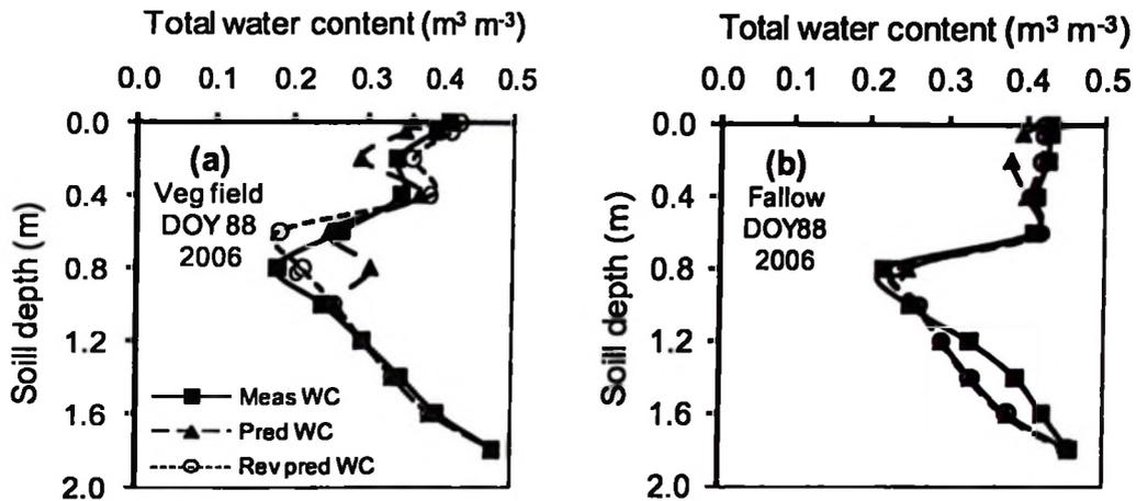
**Fig. 7.7.** Comparison of predicted soil water content from the original and revised (rev) SHAW model for: (a) vegetated fields (oats with berseem clover cover crop) and (b) continuous fallow treatments on March 29, 2006.
