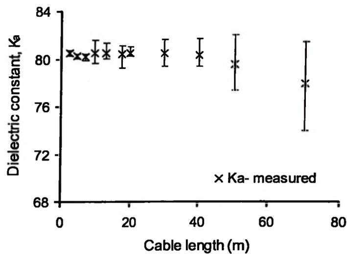
**Fig. 3.4. Variability of the measured dielectric constant of water with increase in cable length. Error bars represent standard errors of measurement.**
