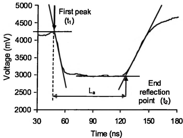
**Fig. 3.1. Typical waveform for a 35-mm TDR miniprobe immersed in pure water and attached to a 2.5-m coaxial cable. The difference between the first peak and the end reflection defines the apparent length,  $L_a$  of the waveguide.**
