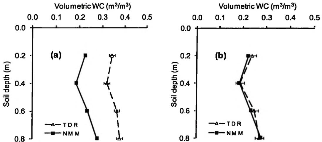
**Fig. 4.1. Comparison of TDR and NMM soil moisture measurements on the cover-cropped treatment at temperature ranges 6.5°C to 2.3°C on November 22, 2005: (a) before temperature correction and (b) after temperature correction. The TDR measurements were taken as average of three replicates.**
