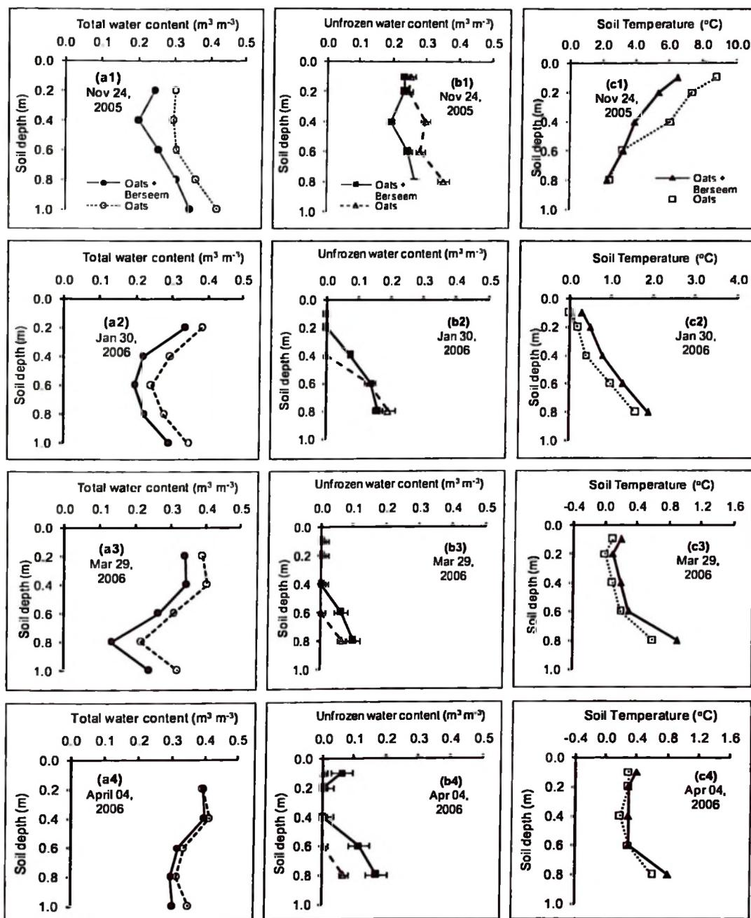
**Fig. 5.4. (a) Total water content (measured with NMM), (b) unfrozen water content (measured with TDR), and (c) soil temperature variation for the oats with berseem clover cover crop and oats alone treatments during: (1) the fall of 2005, and (2) winter and (3, 4) spring of 2006. Error bars for TDR measurements indicates standard errors of three replicate measurements for each soil depth.**
