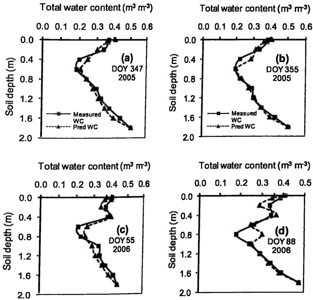
**Fig. 7.1. Measured and predicted total soil water contents at different soil depths in the oats + berseem clover cover crop treatment during: (a and b) the fall in 2005 and (c and d) winter and spring in 2006.**
