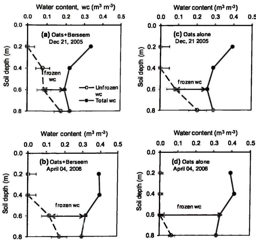
**Fig. 5.5. Partitioning of total water content into frozen and unfrozen phases for the oats with berseem clover cover crop and oats alone treatments during: (a and c) fall freeze-up in December 2005, and (b and d) spring in April 2006. The difference between the two curves represents the amount of soil moisture in the frozen state. Error bars indicate standard errors of measurement for three TDR replicates.**
