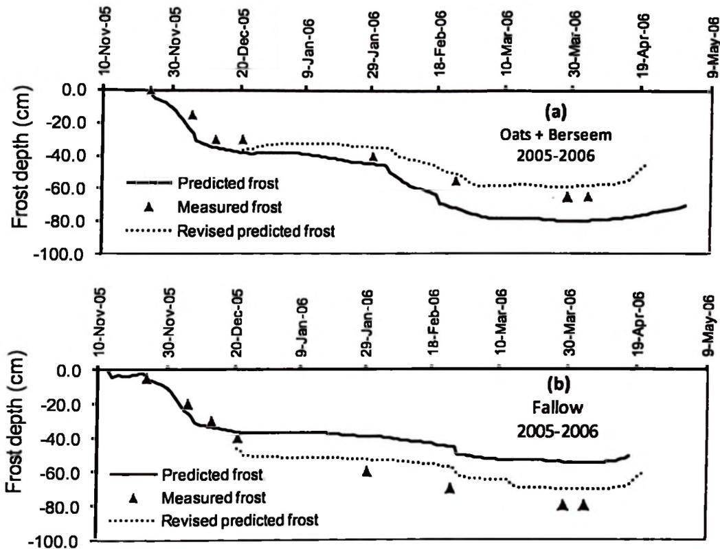
**Fig. 7.8. Comparison of the measured and simulated frost depths from the original and revised Simultaneous Heat and Water (SHAW) models for: (a) vegetated fields (oats with berseem clover cover crop) and (b) continuous fallow treatments in the 2005-2006 seasons. Time Domain Reflectometry (TDR) measurements were used to determine the measured frost depth.**
