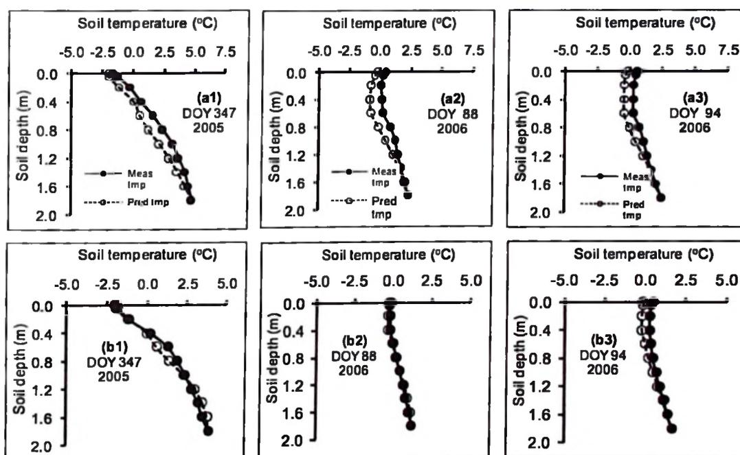
**Fig. 7.3. Measured and predicted soil temperature at different soil depths: (a) in the oats + berseem clover cover crop and (b) in the fallow treatment. The measurements on (a1) and (b1) were during the fall; (a2) and (b2) during winter; and (a3) and (b3) during spring.**
