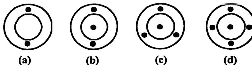
**Fig. 2.1 Commonly used TDR probe rods configurations: (a) two-wire; (b) three-wire; (c) four-wire; and (d) five-wire configuration.**
