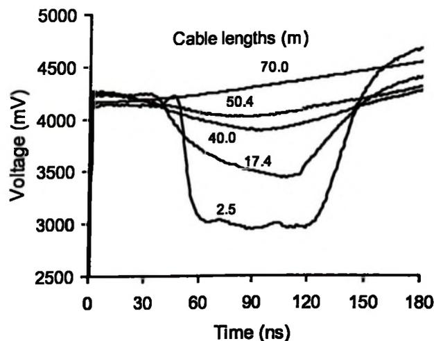
**Fig. 3.2. TDR waveforms for different cable lengths produced using a 35-mm TDR miniprobe immersed in pure water at an average temperature of 20°C.**
