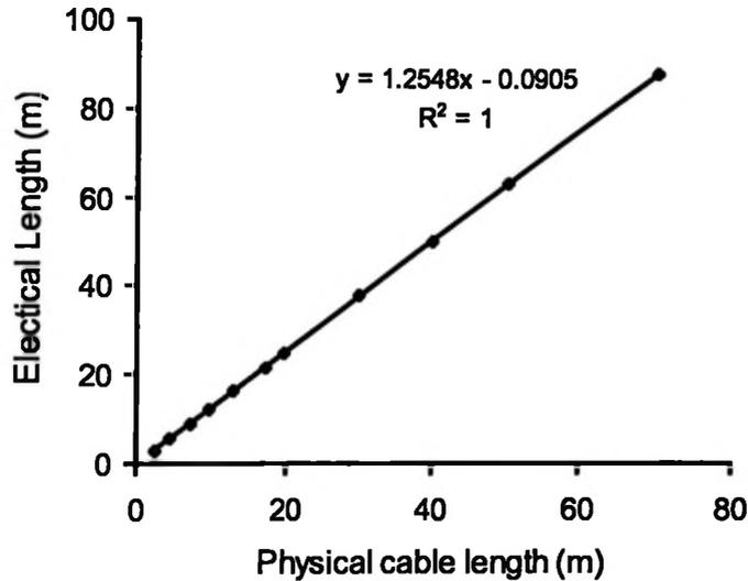
**Fig. 3.5. Comparison of physical and apparent cable lengths for water content measurement.**
