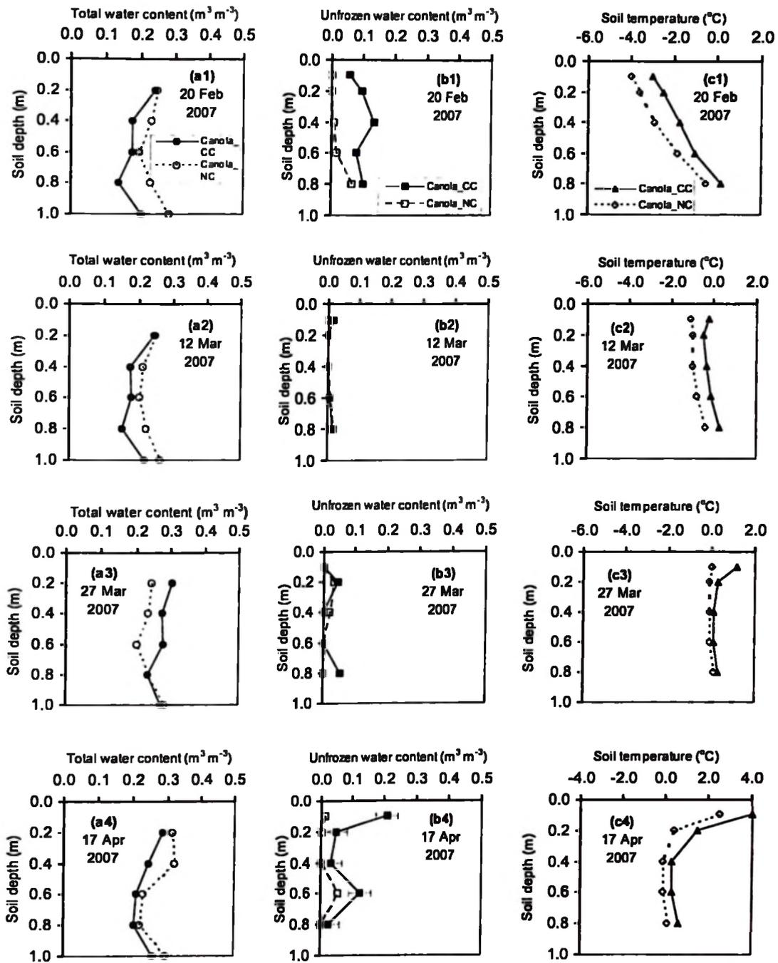
**Fig. 6.7. (a) Total (NMM) water content, (b) unfrozen (TDR) water content, and (c) soil temperature variations with depth for the canola\_CC and canola\_NC treatments during the winter and spring of 2007. Rows 1 to 4 in the figure indicate different sampling dates.**
