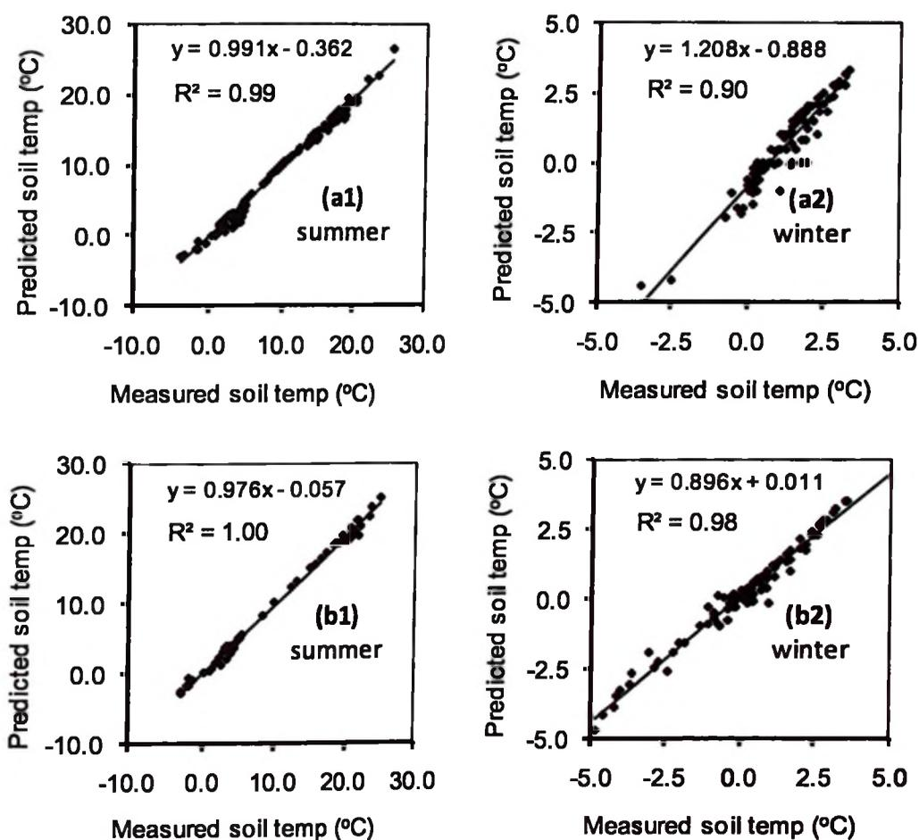
**Fig. 7.5. Scatter plots of estimated versus measured soil temperature profile during the summer of 2005 and winter 2006 for: (a) vegetated fields (oats with berseem clover cover crop) and (b) continuous fallow.**
