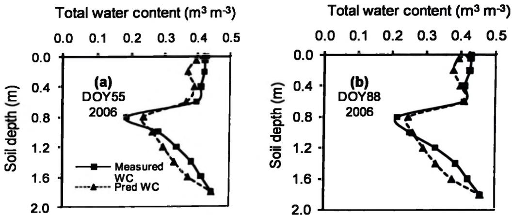
**Fig. 7.2. Measured and predicted total soil water contents at different soil depths in the fallow during: (a) winter on February 24, 2006 and (b) early spring on March 29, 2006. The measured total water contents (WC) were taken using NMM method.**
