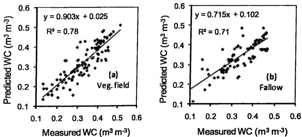
**Fig. 7.6.** Scatter plots of the measured vs. estimated soil moisture, predicted using the revised SHAW model during the winter of 2006 and 2007 for: (a) vegetated fields (oats with berseem clover cover crop) and (b) continuous fallow treatments.
