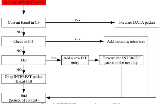
Figure 8: INTEREST packet mechanism in NDN
