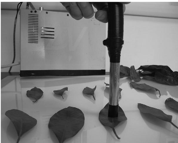
**Fig. 1** – Performing VIS–NIR spectral measurement on citrus leaves.
