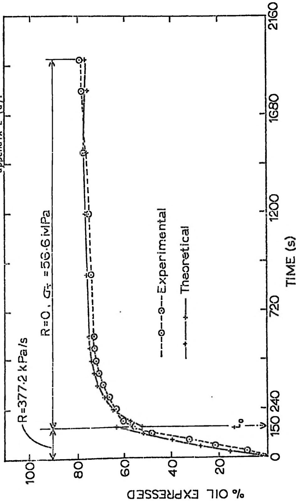
FIG. 41: EXPERIMENTAL AND THEORETICAL RESULTS OF % OIL EXPRESSED AGAINST TIME.
