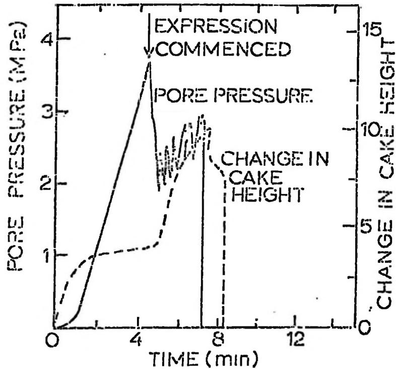
**FIG. 27: VARIATION OF PORE PRESSURE AND CAKE HEIGHT DURING UNDRAINED COMPRESSION WITH OIL EXPRESSION (LEAKAGE) INITIATED DURING THE COMPRESSION. FOR RAPESEED.**
