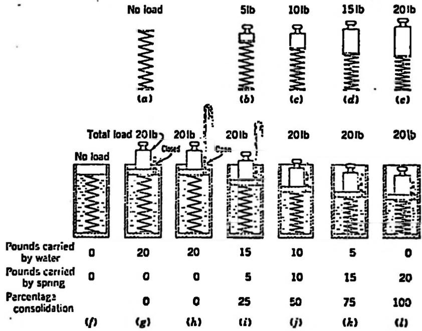
FIG. 4. The piston and spring analogy.
