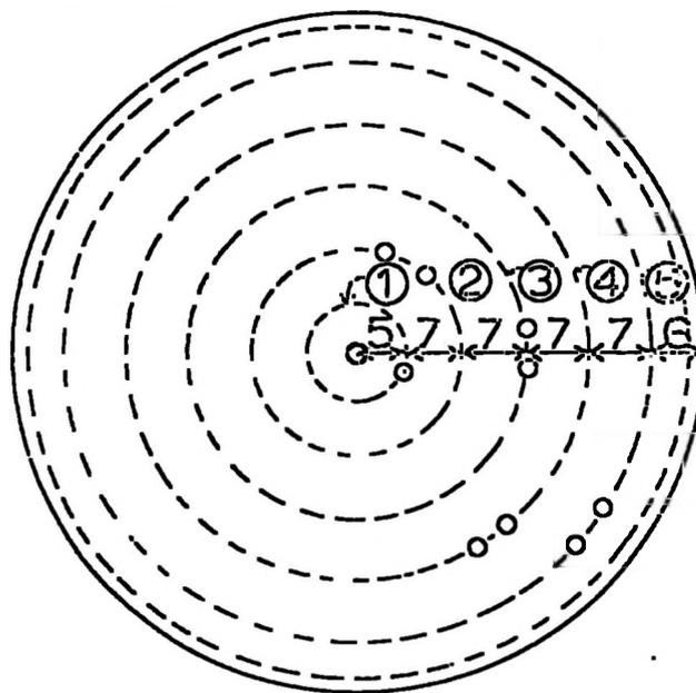
2 mm holes in Circles 1 - 5 at approximately 6 mm distance apart, 6 porous discs used:
