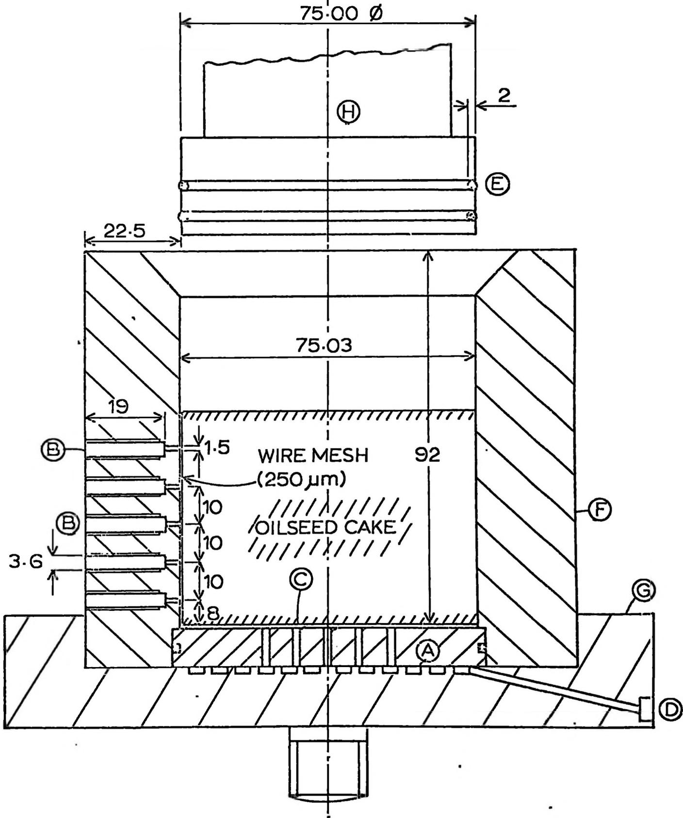
**FIG. 16: POROUS DISCS AT BASE OF CYLINDER FOR OIL EXPRESSION RIG (FIG. 16)**
