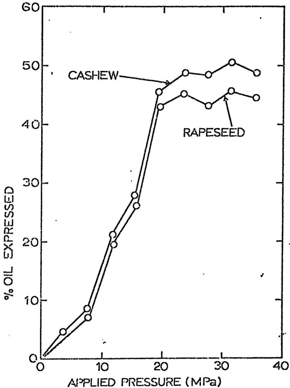
**FIG. 8:** EFFECT OF APPLIED PRESSURE ON OIL EXPRESSION. Load raised from zero at a constant straining rate of 2mm/min. Until desired pressure and immediately cut off. Oil expressed determined by weighing cake after expression.
