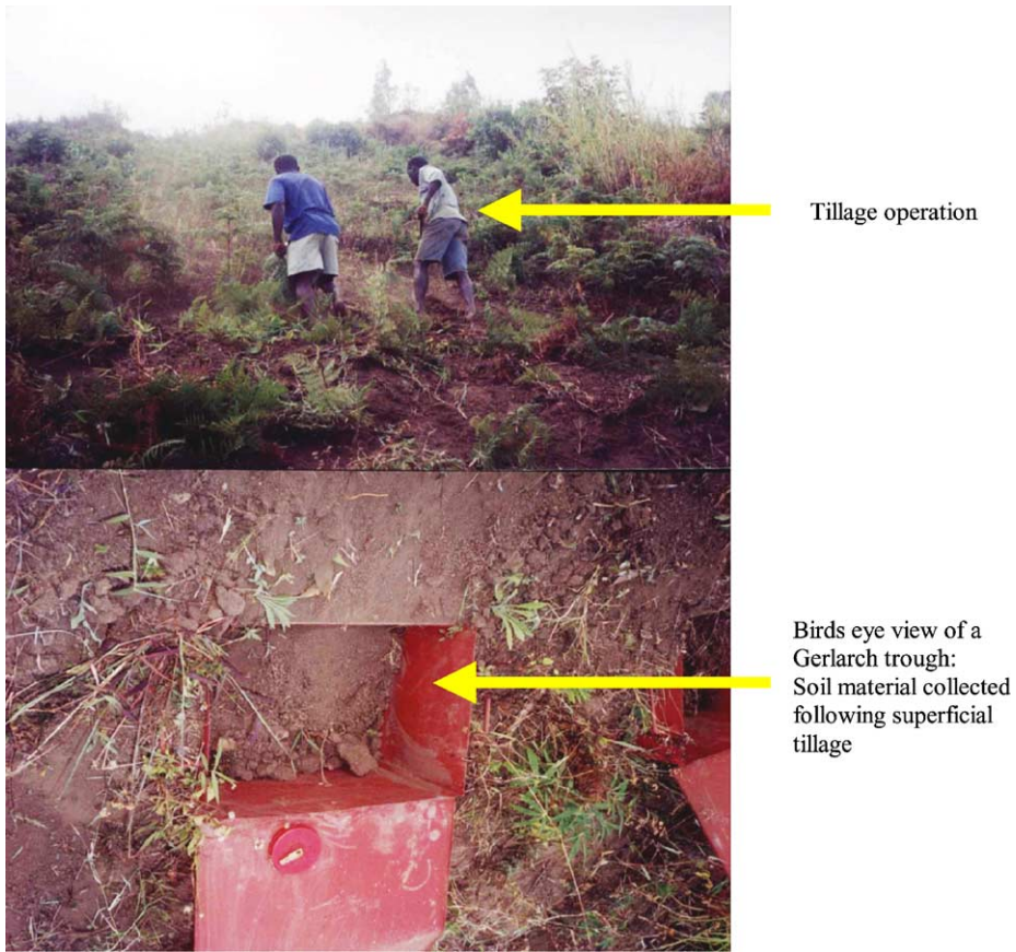
Fig. 4. Measurement of soil translocation due to superficial manual tillage by Gerlarch trough method.
