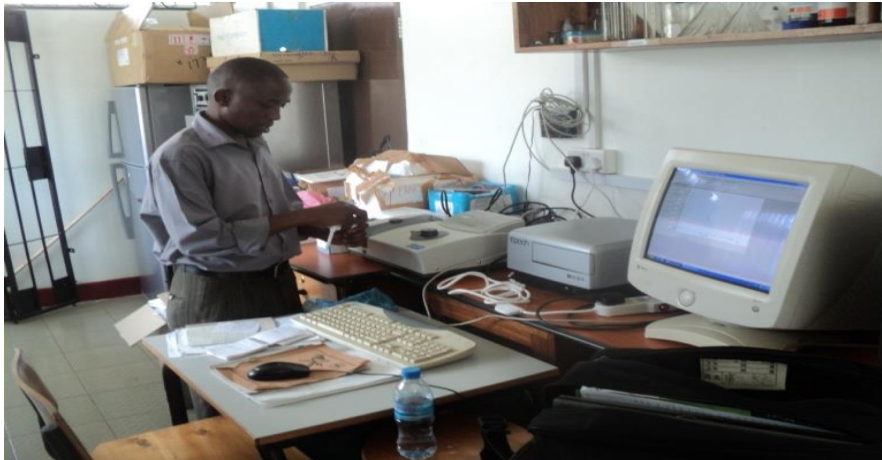
Plate 3: Researcher Analyzing AChE and BuChE in the Blood of O. niloticus Using UV-Vis Spectrophotometer.
