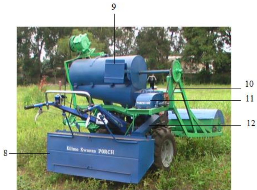
Figure 7: PORCH hitched to a power tiller viewed from the rear
