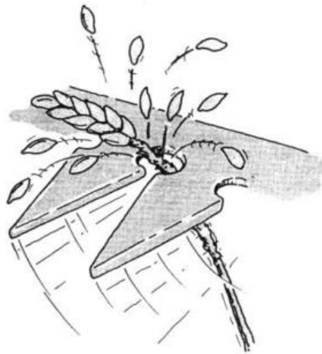
Figure 4: Stripping action of Silsoe stripping device (Source: Horio, 2012)
