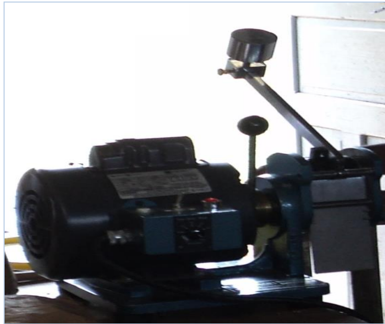
Plate 1: Grainman Rice Miller with lever arm press during dehulling rough grain rice
