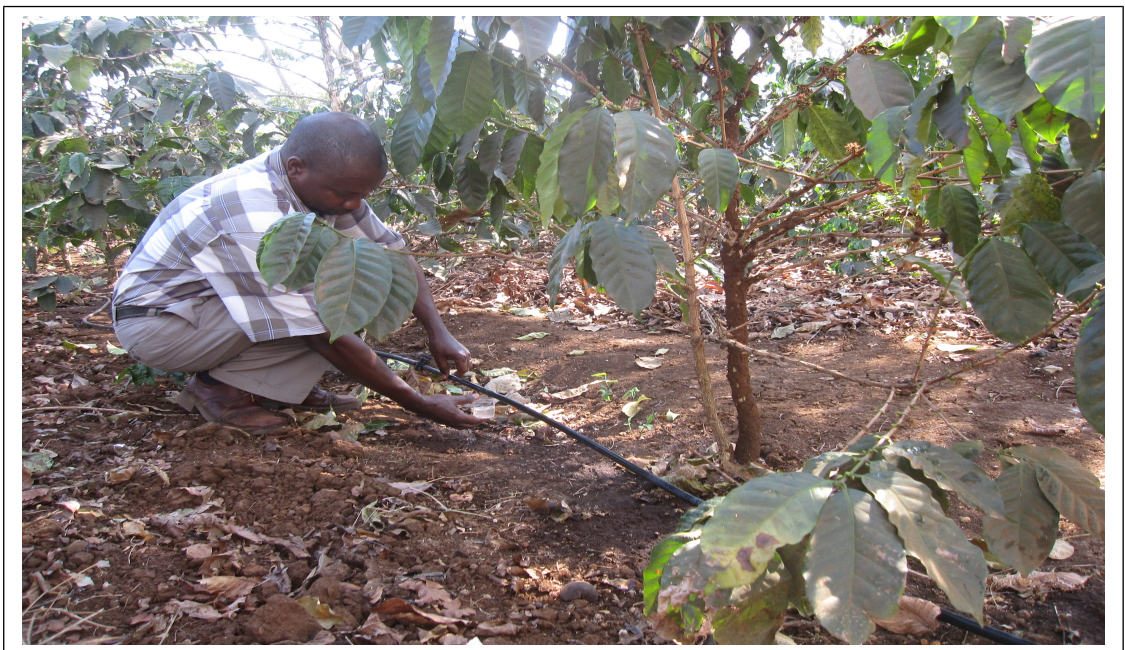
Plate 3: Measuring application rate using catch cans
