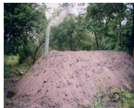
Figure 3: Improved Basic Earth mound Kiln (IBEK)
