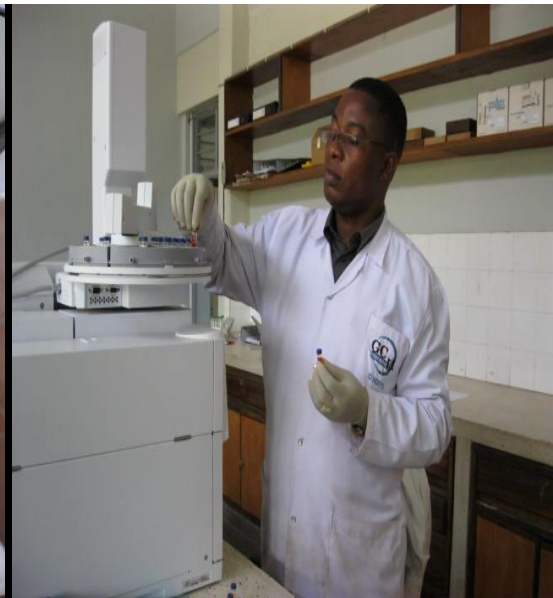
Photo 4: Loading sample in an autosampler GC-MS for residues determination
