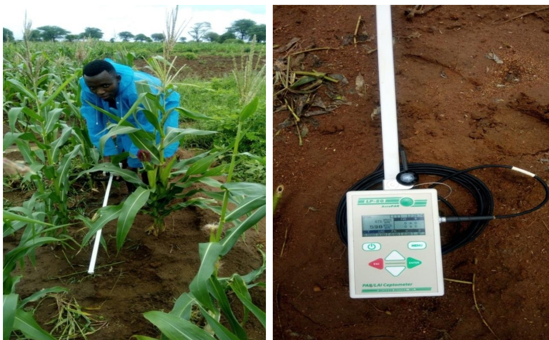
Plate 3: Leaf Area Index (LAI) recorded directly by using an AccuPAR PAR/LAI Ceptometer Model LP-80 device (Credit photo: Elvis Jonas, 2018).
