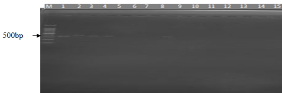
Figure 3.7: Agarose gel 2% eletrophoresis of PCR amplification products of Pyricularia oryzae genomic DNA using primers ACT - 512 F and ACT - 783 R. M = Ladder (1.5kb) and number 1-15 on the jelly are the number of lanes where samples were loaded
