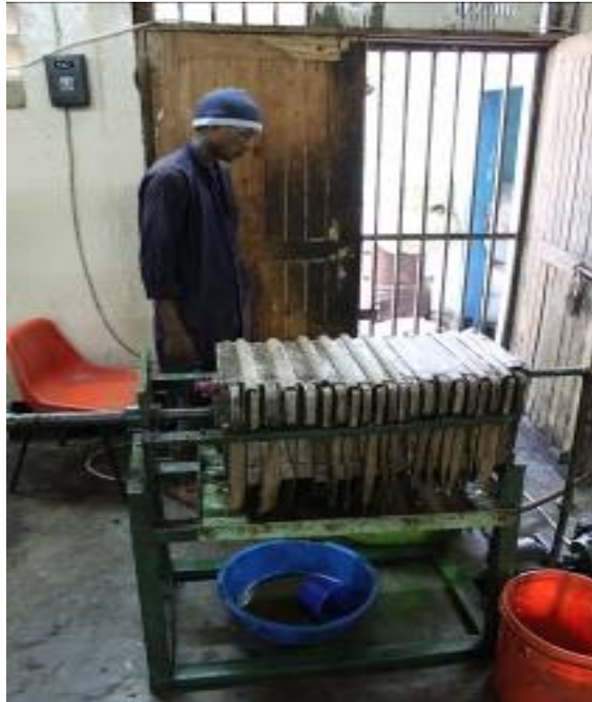
Figure 3: Filtration (cloth press) at DILIGENT Company
