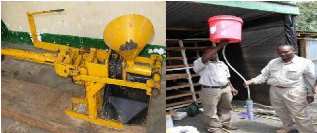
Figure 5: Hand press Machine and Gravity filtration system
