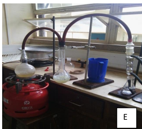
Plate A: Cassava farm; Plate B: Packages of collected cassava samples; Plate C&D: Preparation of cassava solution; Plate E: Steam distillation of sample solution to obtain HCN solution; Plate F: Alkaline titration of HCN solution
