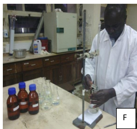
Plate A: Cassava farm; Plate B: Packages of collected cassava samples; Plate C&D: Preparation of cassava solution; Plate E: Steam distillation of sample solution to obtain HCN solution; Plate F: Alkaline titration of HCN solution
