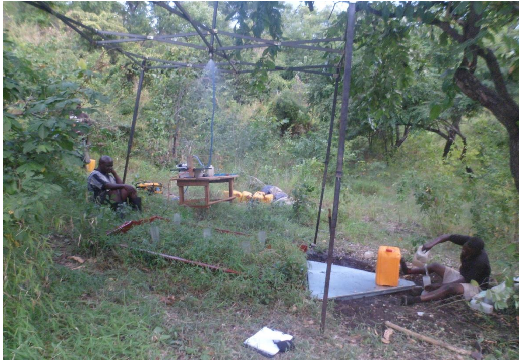
Plate 3: Performing a rainfall simulation experiment at Mvuha sub-catchment
