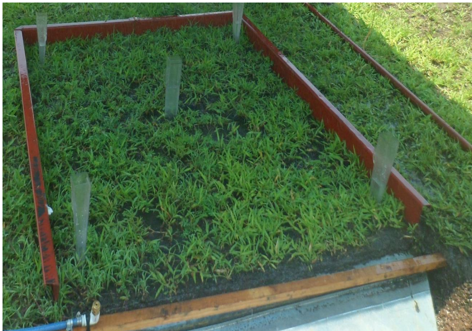
Plate 2: Runoff collection plot with rain gauge installed
