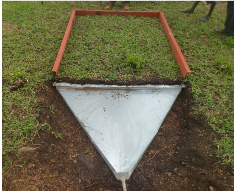
Plate 1: Runoff collection plot at Mvuha sub-catchment
