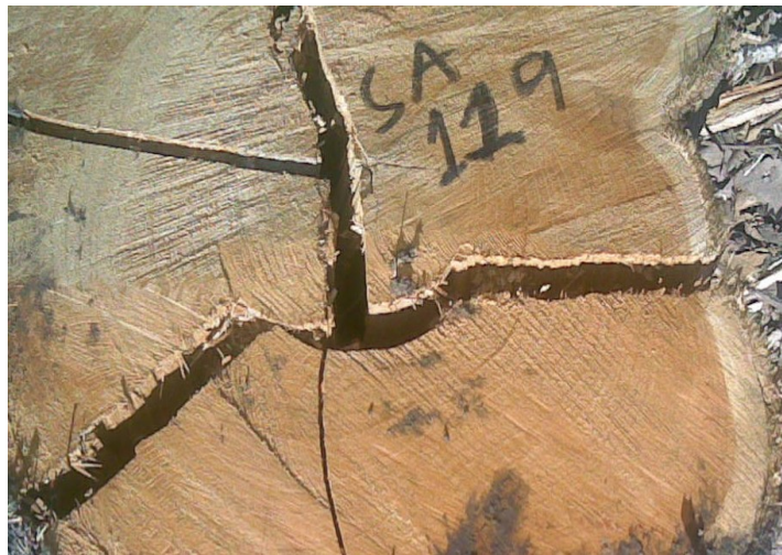
Figure 2: Splits at one end of a teak log at Mtibwa plantation forest
