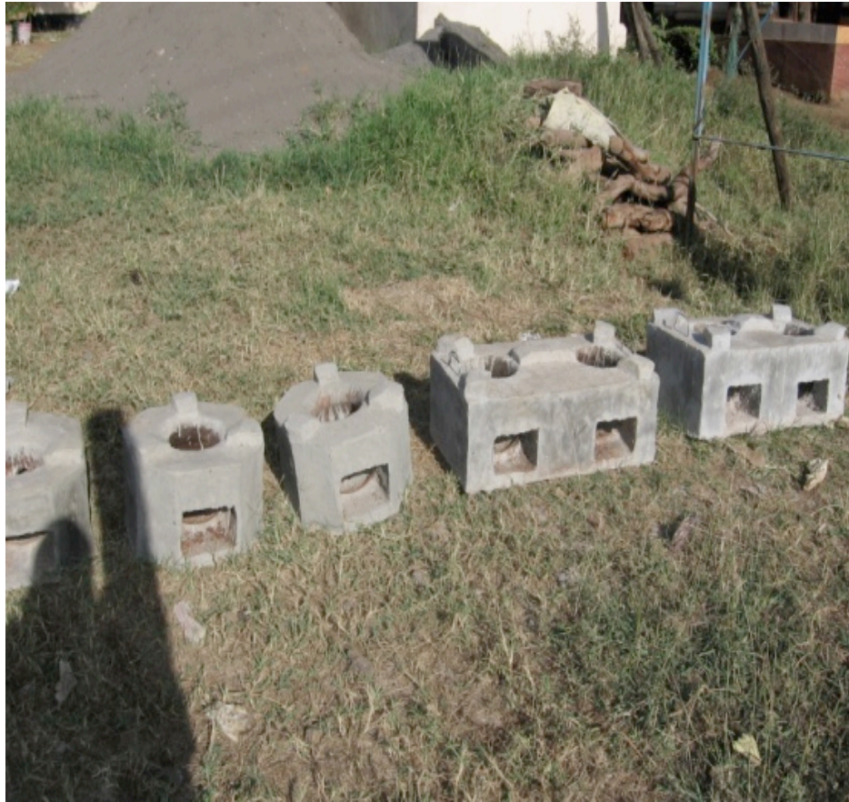
IMAGE 2. ICS without chimneys. Locally made ( Dr. Mwasha Store ).
