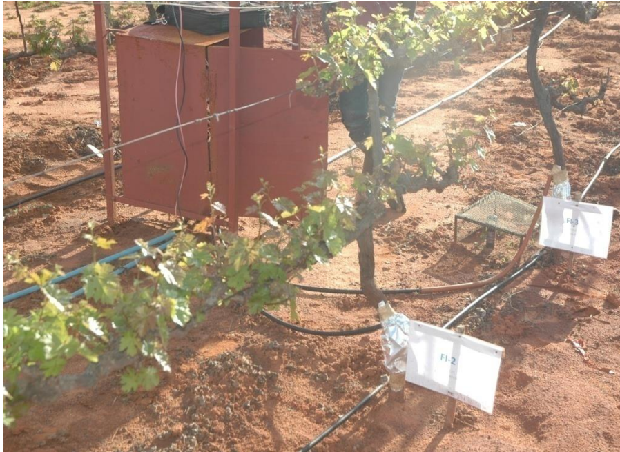
Connections of sap flow probes to the logger
