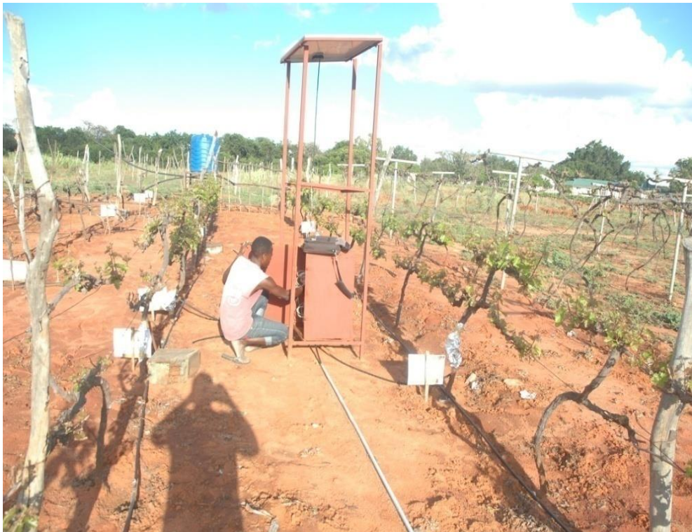
Figure 2.2: Sap flow measuring set, the data logger, a battery and heater switches are caged for safety and shading from weather
