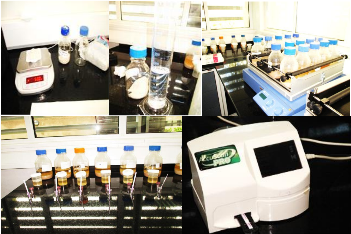
Figure 6: Laboratory procedures used in this study for quantification of aflatoxins and fumonisins by AccuScan-Pro® III reader
