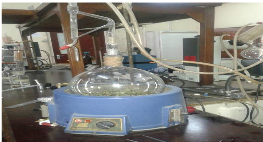
Figure 4: Clavenger apparatus for steam distillation used for extraction of essential oils
