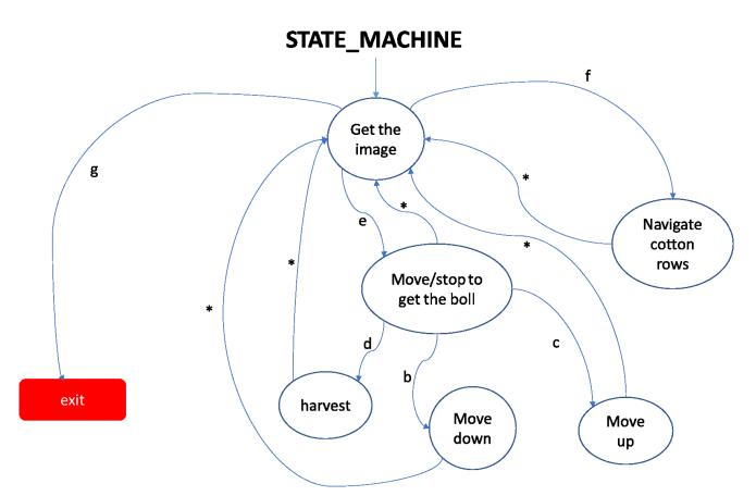
Figure 8. State Machine Diagram of the rover states and transitions
