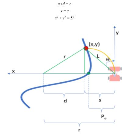
Figure 4. The geometry of the Pure Pursuit algorithm
