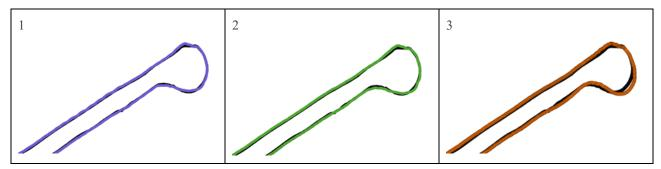
Figure 12. Path tracking of the prescribed path (black). The blue, green and orange path tracking is the GPS generated path of the rover when following the rows using prescribed path (black)
