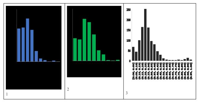
Figure 13. The distribution of absolute errors is clearly skewed to the left. It shows that the rovers were navigating along the rows safely with less than 30 cm absolute error.
