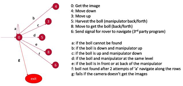
Figure 9. Linear transformation of the State Machine Diagram (Fig 8) of the rover states and transitions
