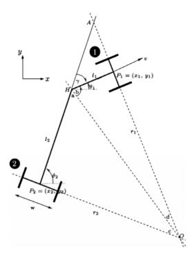
Figure 5. The geometry of the center-articulated rover while turning.  $\mathbf{r}_1$  is the distance from the origin of the turning circle O (Corke & Ridley, 2001)
