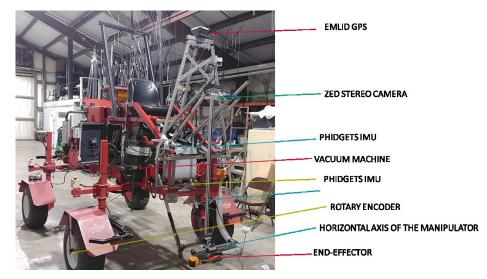
Figure 1. The research red rover with manipulator and sensors attached in front of the rover implemented for this study
