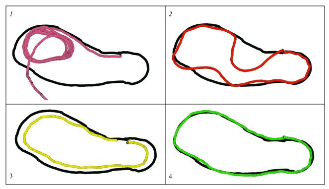
Figure 10. Performance of the rover when the (1)ROS updates are so high (10Hz), (2)Short look ahead distance (1m), (3) no path error correction is applied and (4)successful path tracking when look-ahead is 3m, path error is 1.5 times path error and ROS updates at 1Hz
