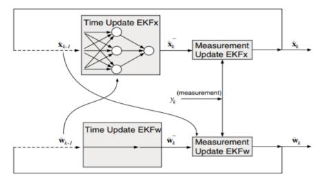
Figure 3. The dual extended Kalman filter. The algorithm consists of two EKFs that run concurrently. The top EKF generates state estimates and requires  $\hat{w}_{k-1}$  for the time update. The bottom EKF generates weight estimates and requires  $\hat{x}_{k-1}$  for the measurement updates (Wan and Nelson, 2001).
