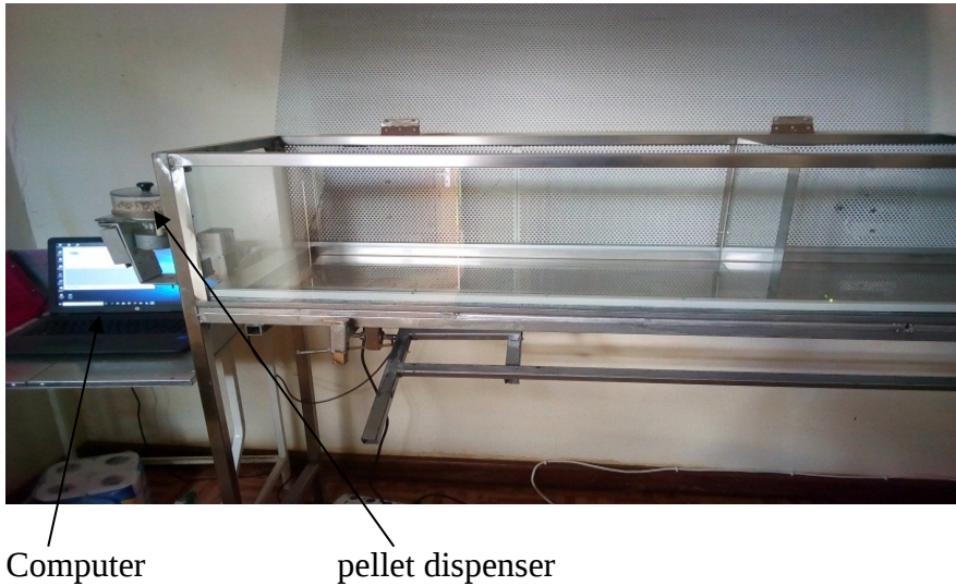
Figure 3: Fully automated line cage system.
