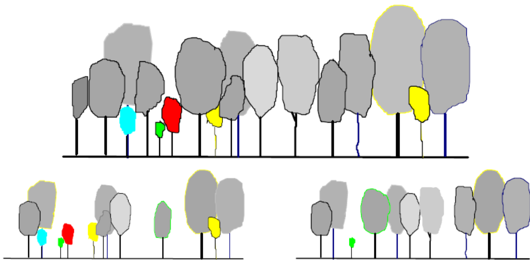
Figure 1: Schematic representation of two different thinning operations in an even-aged beech stand. Above: stand before the thinning; below left: after a heavy high thinning; below right: after a moderate low thinning
