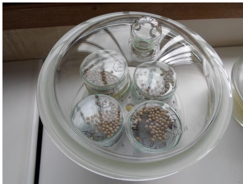
Plate 2: Moisture content determination by oven dry method
