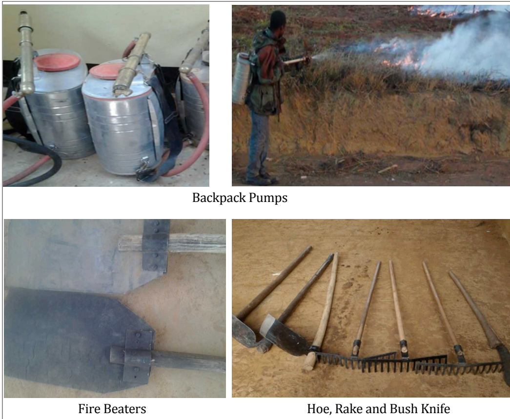
Figure 4.3. Examples of fire fighting equipment (A photo from SAO hill forest plantation in Tanzania)
