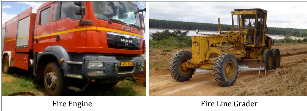
Figure 4.4. Examples of mechanical equipment used for fire fighting (A photo from SAO hill forest plantation in Tanzania)
