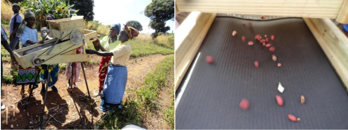
Figures 10 & 11: CTI's Incline Belt Sorter - Good kernels roll down, broken kernels ride up the belt
