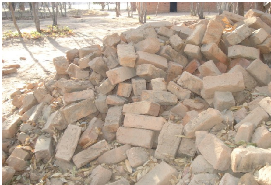
Plate 1: Burnt bricks on site at Mapogoro Village
